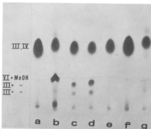
FIG. 2. TLC System A. a = Adduct III, 3 days, 170 C, with and without maleic anhydride (MA); b = ergosteryl acetate (EA)-MA reaction products refluxed 4 hr in methanol; c = adduct III refluxed overnight in methanol; d = crude EA-MA adduct III; e = purified adduct III; f = 22,23-dihydroadduct IV; g = 6,7,22,23-tetrahydroadduct. III, IV, V = see Scheme 1.
